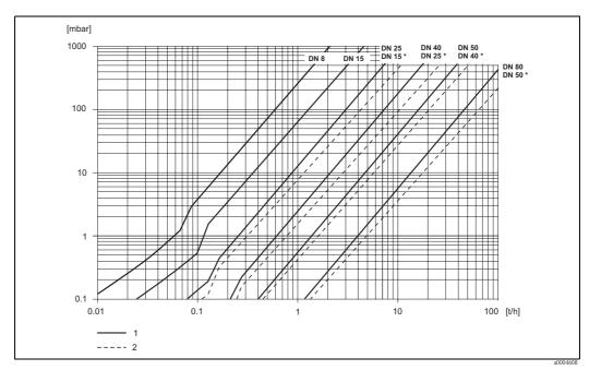
Fig. 41: Pressure loss diagram for water
