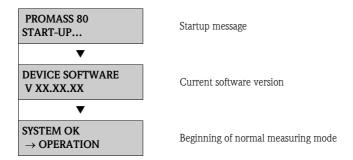
Normal measuring mode commences as soon as startup completes. Various measured value and/or status variables appear on the display (HOME position).g
