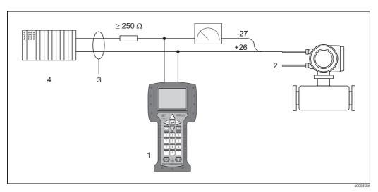
Fig. 21: Electrical connection of HART handheld terminal
