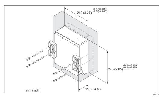
Fig. 14: Panel installation (wall-mount housing)
