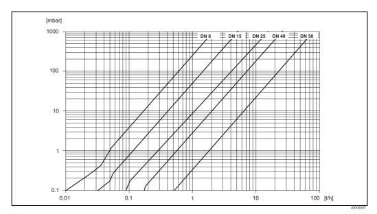
Fig. 40: Pressure loss diagram for water
