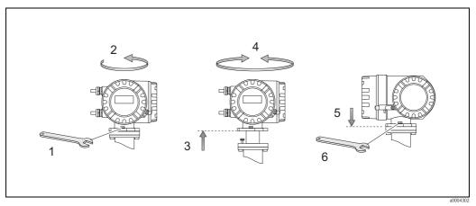
Fig. 11: Turning the transmitter housing (aluminum field housing)
