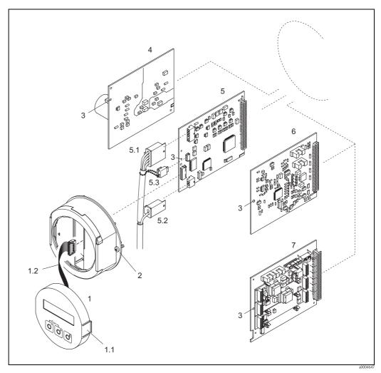
Fig. 32: Field housing: removing and installing printed circuit boards
