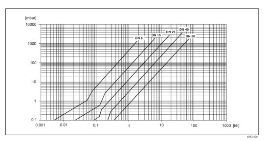
Fig. 38: Pressure loss diagram for water
