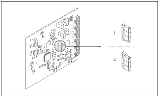
Fig. 28: Configuring the current output (I/O board)
