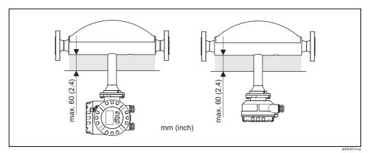
Fig. 10: In the case of the Promass F high-temperature version, a maximum insulation thickness of 60 mm (2.4") must be observed in the area of the electronics/neck.
