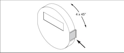
Fig. 16: Turning the local display (field housing)
