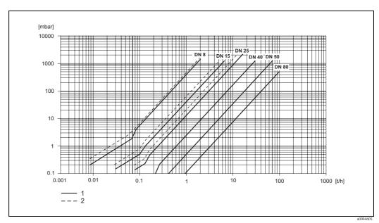
Fig. 37: Pressure loss diagram for water
