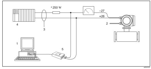
Fig. 22: Electrical connection of a PC with operating software
