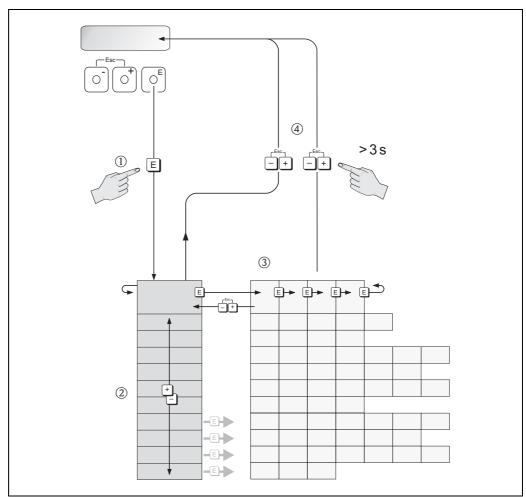
Fig. 25: Selecting functions and configuring parameters (function matrix)
