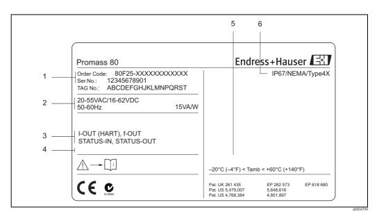
Fig. 2: Nameplate specifications for the "Promass 80" transmitter (example)
