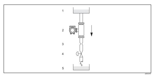
Fig. 7: Installation in a vertical pipe (e.g. for batching applications)
