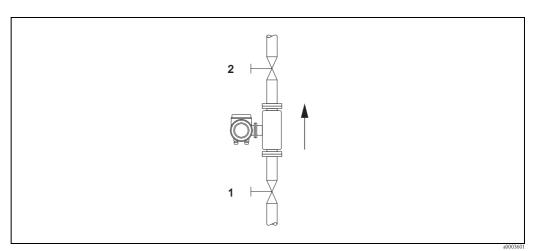
Fig. 30: Zero point adjustment and shutoff valves
