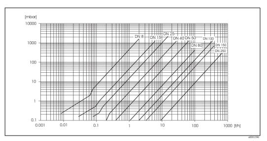
Fig. 36: Pressure loss diagram for water
