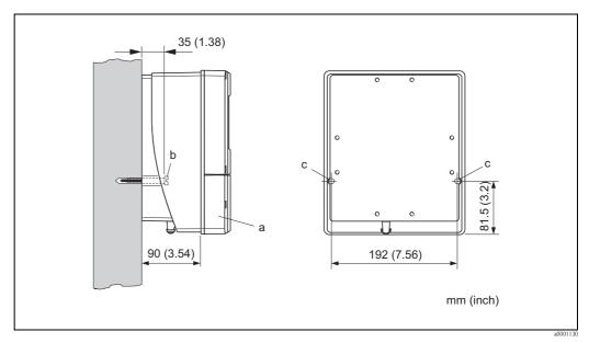
Fig. 13: Mounted directly on the wall
