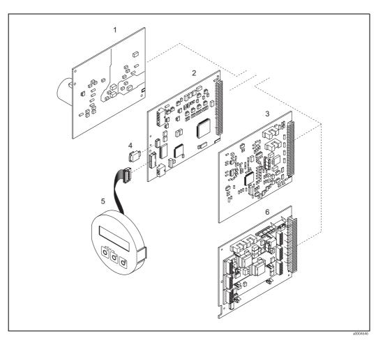
Fig. 31: Spare parts for transmitter Promass 80 (field and wall-mount housing)
