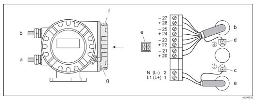
Fig. 18: Connecting the transmitter (aluminum field housing). Cable cross-section: max. 2.5 mm<sup>2</sup>
