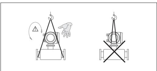
Fig. 5: Instructions for transporting sensors with  $> DN 40 (> 1\frac{1}{2})$ "
