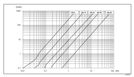
Abb. 42: Pressure loss diagram for water
