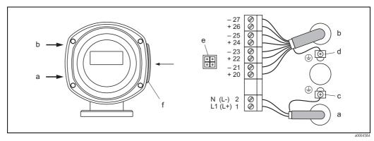
Fig. 19: Connecting the transmitter (stainless steel field housing); cable cross-section: max. 2.5 mm<sup>2</sup>
