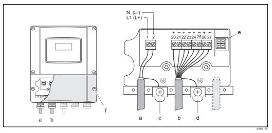
Fig. 20: Connecting the transmitter (wall-mount housing); cable cross-section: max. 2.5 mm<sup>2</sup>
