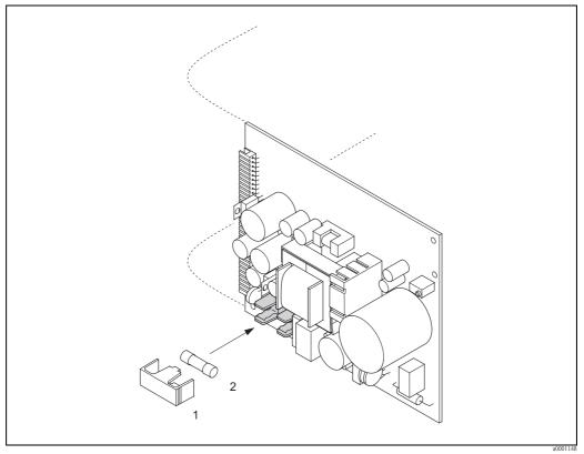
Fig. 34: Replacing the device fuse on the power unit board
