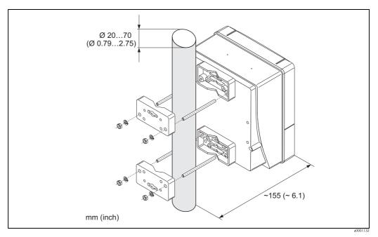
Fig. 15: Pipe mounting (wall-mount housing)
