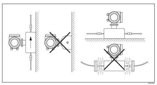
Fig. 8: Vertical and horizontal orientation (Promass A)
