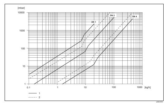
Fig. 39: Pressure loss diagram for water
